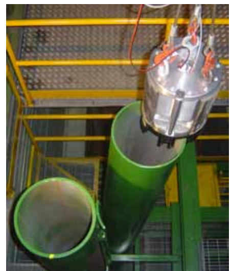
Fig. 4 Insertion of the fixing mechanism in an inclined DSU cell mock-up.
